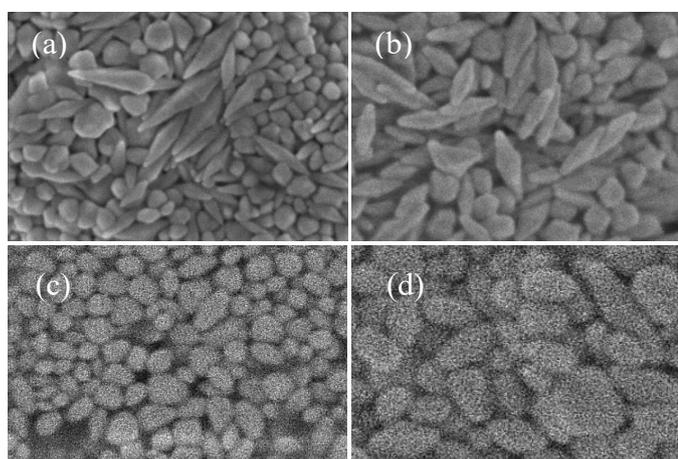
**Fig. 2.** Morphology FESEM of A-GNBPs (a) 0.5 hour (b) 1 hour (c) 2 hours (c) 3 hours
