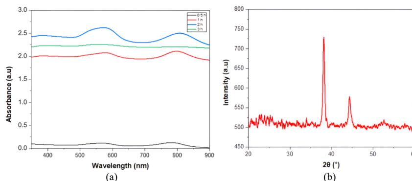
**Fig. 1.** (a) UV-Vis absorption spectrum of Ag-GNBPs sample with growth time variation (b) XRD Spectrum
